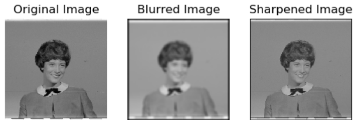
Figure 7.5 – Performing operations with kernels
