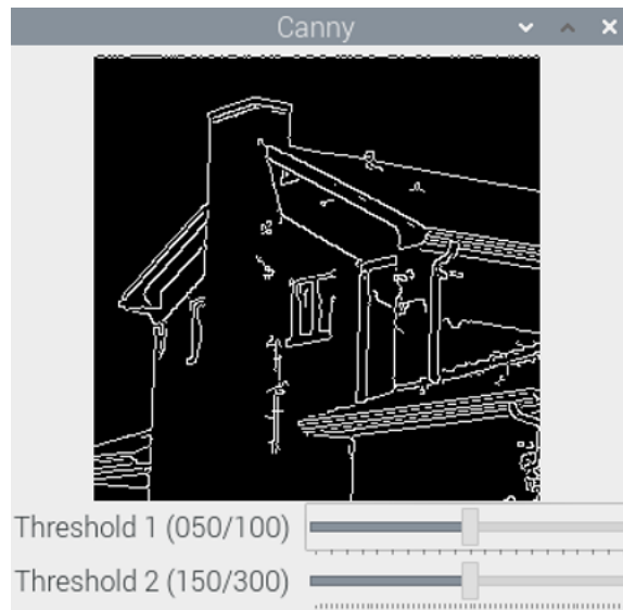
Figure 8.4 – The output of the Canny edge detection algorithm with trackbars
