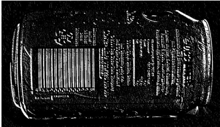
Figure 11.7 – Difference between horizontal and vertical Sobel derivatives
