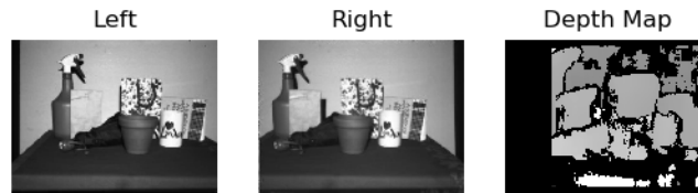
Figure 9.7 – Estimation of depth from the disparity map
