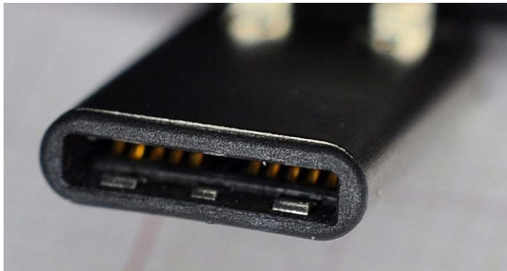
Figure 1.11 – USB Type-C pin
