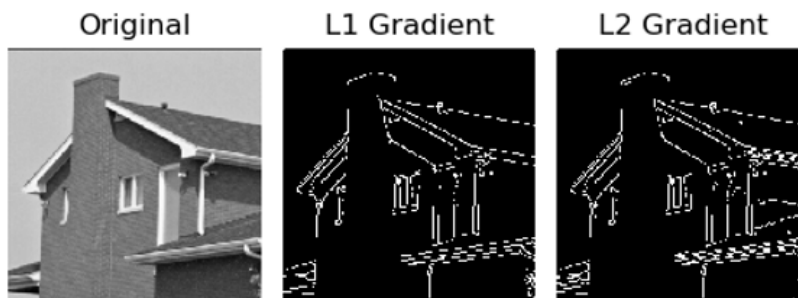
Figure 8.3 – The output of Canny edge detection
