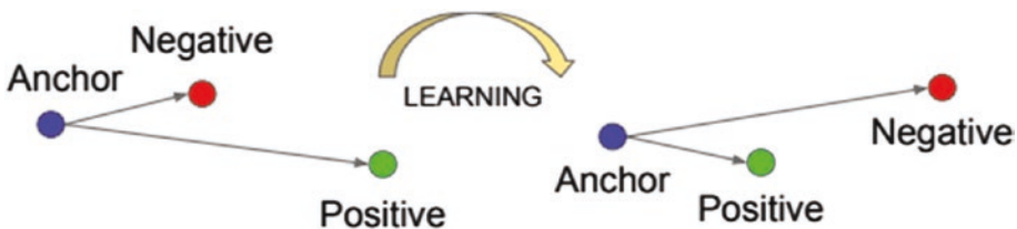
Figure 8-3. The triplet loss minimizes the distance between an anchor and a positive, both of which have the same identity, and it maximizes the distance between the anchor and a negative of a different identity. (Source: FaceNet, https://arxiv.org/pdf/1503.03832.pdf .)
