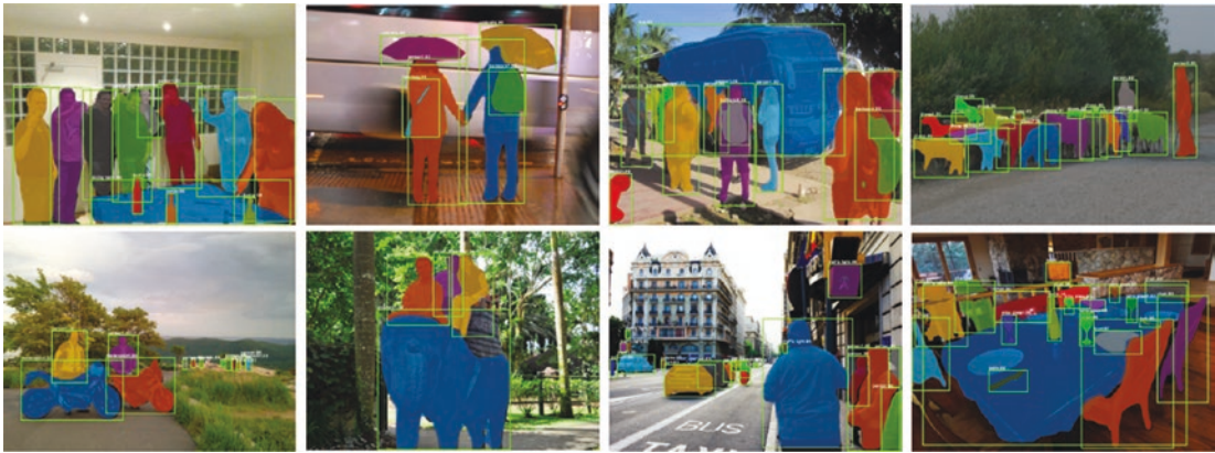
Figure 6-9. Display of images with bounding boxes and masks (image source: Ross Girshick et al.)
