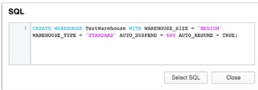
Figure 3-3. Show SQL will display the SQL code that can be used in a script. In this example, AUTO_SUSPEND automatically translates the minutes entered into the Create Warehouse dialog into seconds
