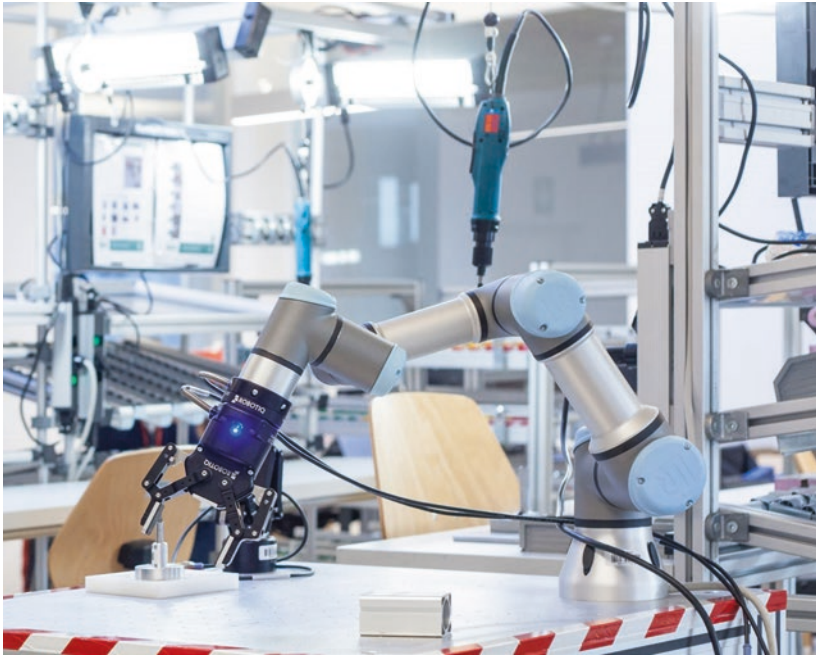
Fig. 12.1 A collaborative robot (UR3 model) in a shared workspace (Source Smart Mini Factory, unibz [Reproduced with permission from Smart Mini Factory Lab, unibz])
