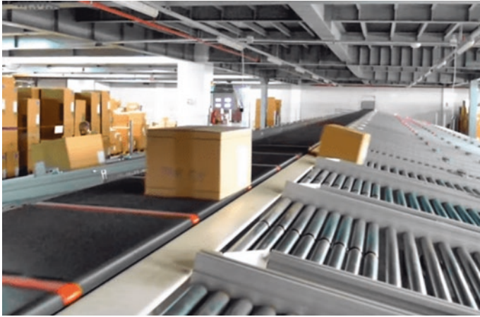
Fig. 7.5 Cross belt sorter (Reproduced with permission from University of Chiang Mai, Department of Industrial Engineering)
