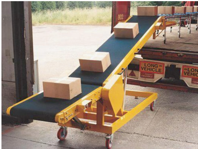
Fig. 7.4 Truck Loading/unloading conveyor systems (Reproduced with permission from University of Chiang Mai, Department of Industrial Engineering)
