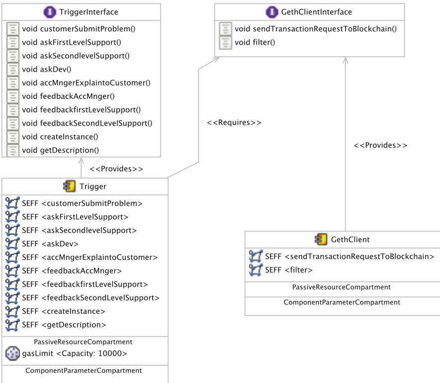
Fig. 10.2 PCM repository diagram showing connected components and the operations provided by their interfaces. © 2017 by the Commonwealth Scientific and Industrial Research Organisation, reprinted with permission
