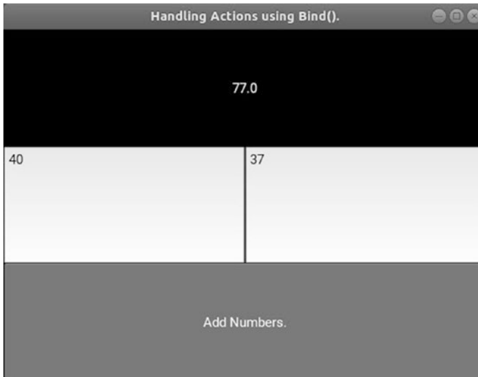
Figure 8-11. Application UI that adds two numbers and displays the result on a Label widget
