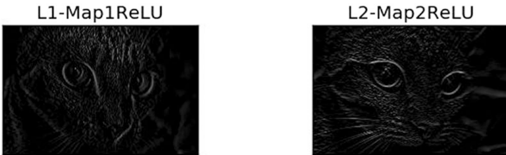
Figure 5-33. ReLU layer output applied to the output of the first conv layer
