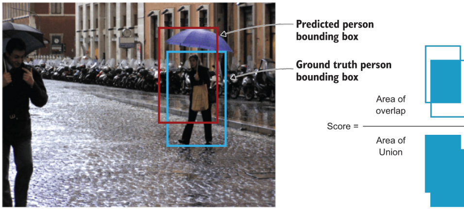
Figure 7.5: IOU score is the overlap between the ground truth bounding box and the predicted bounding box.
