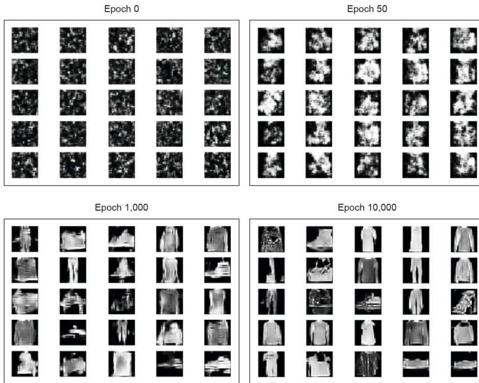
Figure 8.24: Outputs of the GAN Generator after 0, 50, 1000, and 10000 epochs.
