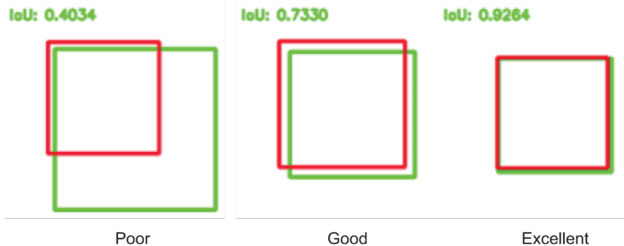
Figure 7.6: the higher overlap (IOU) between the two bounding boxes, the better.
