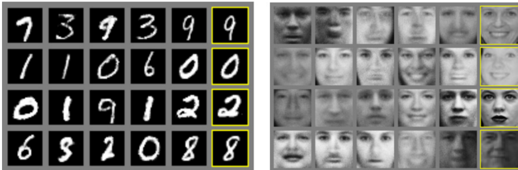
Figure 8.1: Illustration of GANs abilities by Ian Goodfellow and co-authors. These are samples generated by Generative Adversarial Networks after training on two datasets: MNIST and TFD. For both, the rightmost column contains true data. This shows us that the produced data are really generated and not only memorised by the network. (source: "Generative Adversarial Nets" paper).
