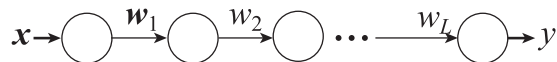
Figure 6.28. An example of an ANN model with only one node at every hidden layer.
