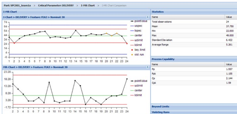
Figure 16.1 An example of a control chart tracking individual measurements (upper chart tracks the measurements, lower chart their moving range representing variability). The right panel provides summary statistics. Source: Figure from SPCLive system by KPA Ltd.
