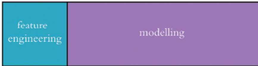
Figure 1-13 Feature engineering—the transformation of raw data into thoughtfully-transformed input variables—often predominates the application of traditional machine learning algorithms. In contrast, the application of deep learning often involves little to no feature engineering, with the majority of time spent instead on the design and tuning of model architectures.
