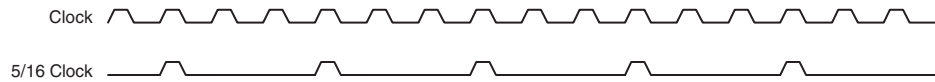
Figure 3.46 Timing Diagram Illustrating the 5/16 Output Frequency for a 4-bit Binary Rate Multiplier
