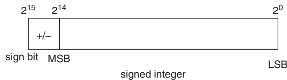
Figure 6.12 Format of a 16-bit Signed Integer
