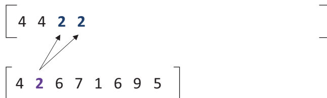
Figure 7-50. The next entry is repeated twice to form the next two entries in the output vector of the upsampling operation
