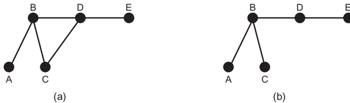
Figure 4.6 In the left graph, a cycle exists between vertices B, C, and D, so it is not a tree. In the right graph, the edge connecting C and D has been pruned, so the graph is a tree.
