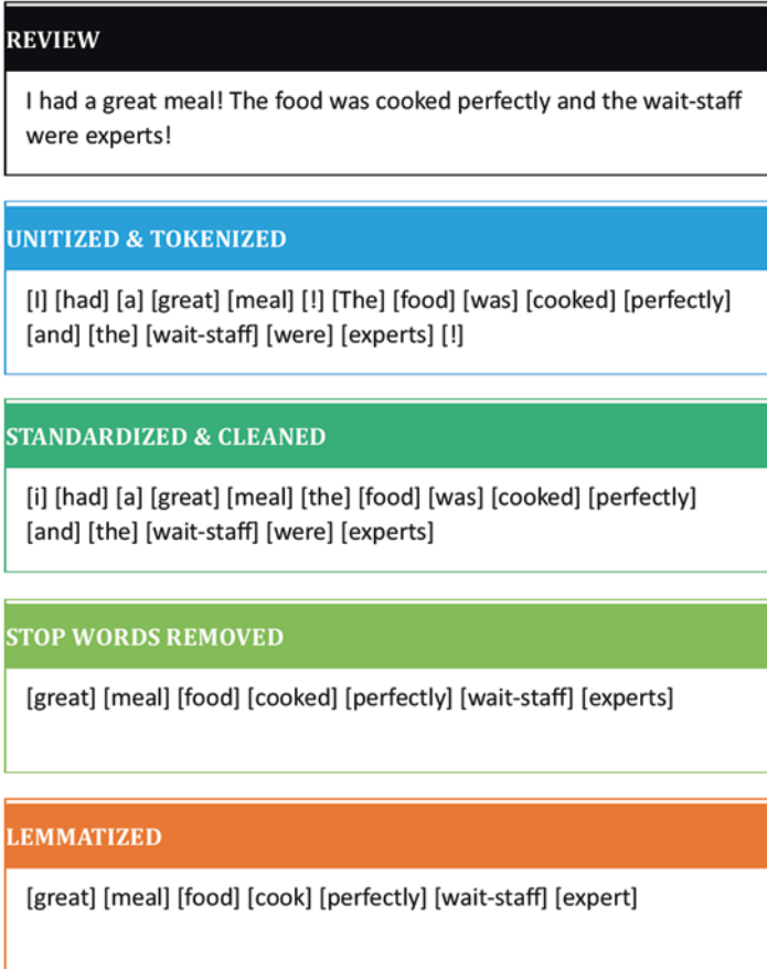
Fig. 10.3 Positive review example: text preparation and preprocessing
