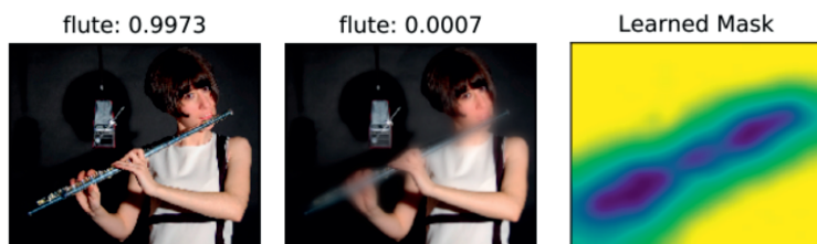
Figure 11.8 Image mask showing what a CNN detects and classifies as a flute, from the paper “Interpretable explanations of black boxes by meaningful perturbation,” by Ruth Fong and Andrea Vedaldi ( arxiv.org/abs/1704.03296 ). When the flute area is blurred (perturbing the data), the CNN’s accuracy at detecting the presence of a flute drops from 99.7% to less than 0.1%.
