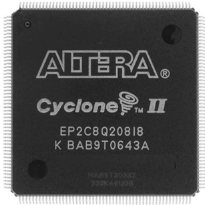
Figure 1.3.1: The programmable logic device “Cyclone II” produced by Altera Corporation.
