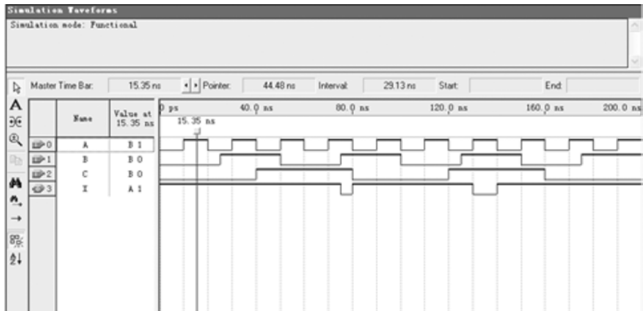
Figure 10.5.4: The output waveform in relation to the inputs after the functional simulation.
