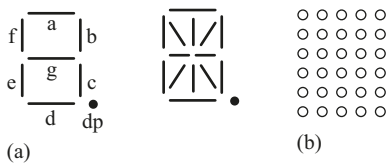
Figure 4.4.18: Illustration diagram of segment display (a) and dot-matrix display (b).
