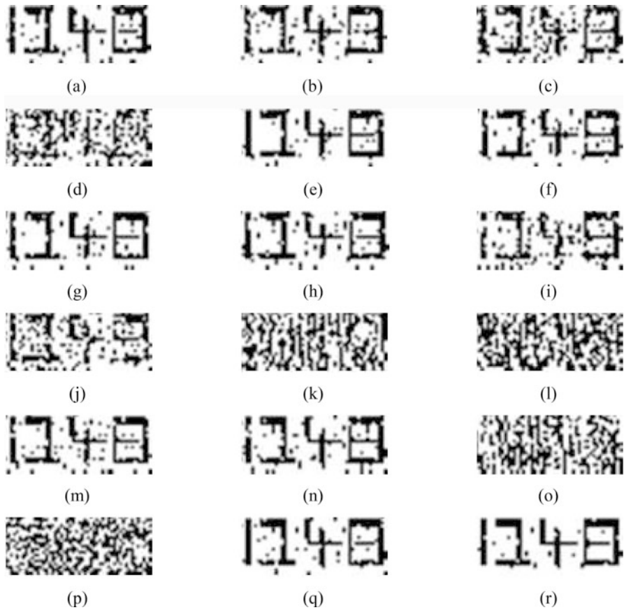
Fig. 9.11 Recovered watermark images 2 from watermarked ear image under various watermarking images: (a–c) for JPEG compression with Q = 90, 80, 70 , respectively, (d) Blurring, (e) Sharpening, (f) Gaussian noise ( \mu = 0, \sigma = 0.0001 ), (g) Salt & pepper noise ( \sigma = 0.0005 ), (h) Speckle noise ( \sigma = 0.0004 ), (i, j) Median filter (Size = 3 \times 3, 5 \times 5 ), (k, l) Mean filter (Size = 3 \times 3, 5 \times 5 ), (m, n) GLPF (Size = 3 \times 3, 5 \times 5 ), (o) Flipping, (p) Rotation ( 90^\circ ), (q) Cropping (20%), (r) Histogram equalization
