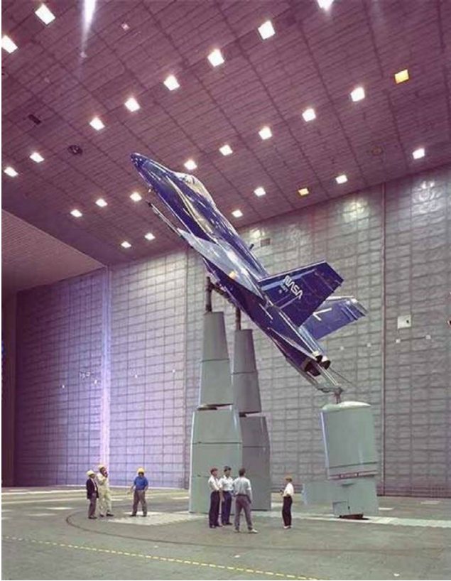
Figure 6.2 A physical model. This full-scale model of an aircraft in a wind tunnel excludes many important properties of the real system, including engines, flight instruments, and a pilot. However, the model is extremely useful for doing what it was designed to do: determining the aerodynamic properties of the aircraft.
