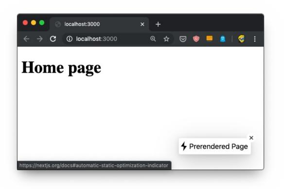
This icon, which is *only visible in development mode* of course, tells you the page qualifies for automatic static optimization, which basically means that it does not depend on data that needs to be fetched at invokation time, and it can be prerendered and built as a static HTML file at build time (when we run npm run build ).
