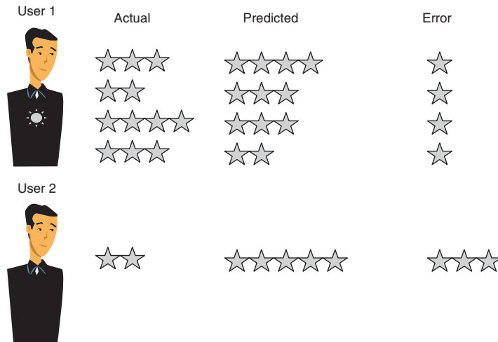
Figure 9.6 Users should have equal weight in the evaluation. Here two users' ratings are shown. User 1 has added four ratings, while user 2 has only added one. If you average all ratings, then the bad experiences of user 2 will drown in the good ratings of user 1.
