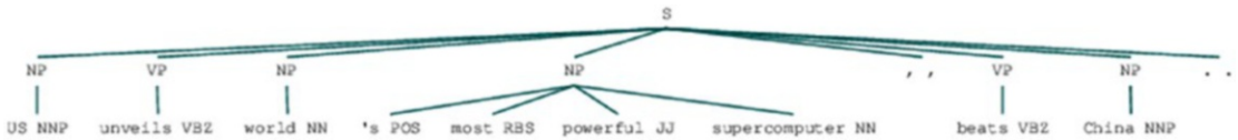
Figure 3-12. Shallow parsed news headline using n -gram based chunking on conll2000 data
