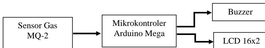
Gambar 1 Diagram blok sistem pendeteksi gas
