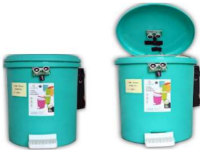
Figure 3. Prototype smart waste container built-in research.
