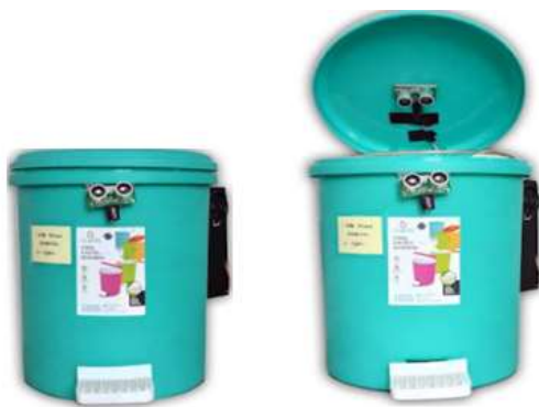
Figure 3. Prototype smart waste container built-in research
