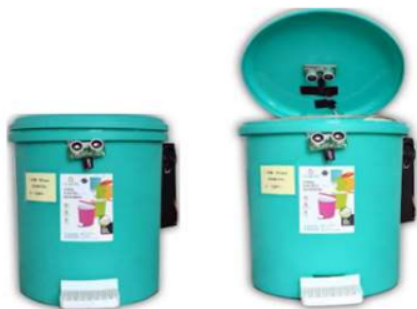
Figure 3. Prototype smart waste container built in research
