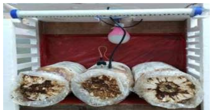
Figure 7. Baglog container with automatic control over water pH, temperature, and humidity of Baglog by developed hardware and software systems
